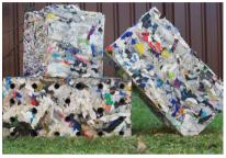
process of heat and compression, creates construction-grade blocks called ByBlocks. The blocks are 22 pounds of plastic which yields a 22-pound construction block. The product is all about creating a zero-waste stream.
